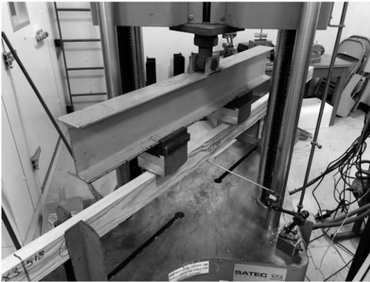
Figure 1. Static bending test setup as per ASTM D198-15.
