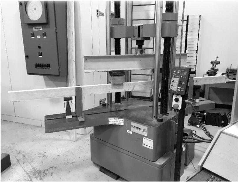
Figure 1. Third-point static bending test fixture per ASTM D 198-15.
